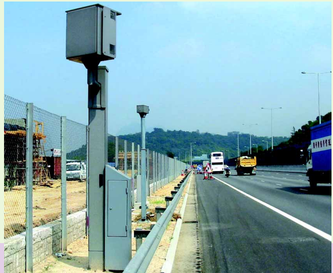
Speed Enforcement Camera along Hong Kong Expressways 設置於快速公路上的偵察車速攝影機
